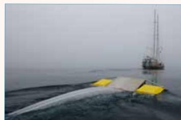
1 - LE FILET MANTA EST TRAINÉ DERRIÈRE LE BATEAU À PETITE VITESSE PUIS REMONTÉ AU BOUT D'UNE HEURE
