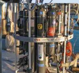
Scientists prepare the rosette, which will go down to a depth of 300 meters to sample elements of marine chemistry (inorganic and organic carbon, nutrients, trace elements, etc.).
