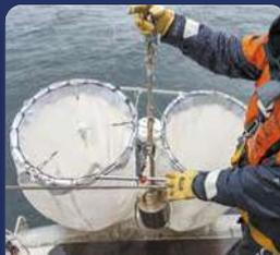
Then they prepare the bongo nets to collect tiny plankton. They filter up to 40,000 liters of seawater in 10 minutes.
