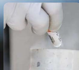
After filtration, each sample is placed in liquid nitrogen at  $-196\text{ }^{\circ}\text{C}$  or refrigerated at  $4\text{-}5\text{ }^{\circ}\text{C}$ .
