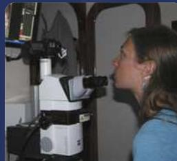
In the dry laboratory, a microscope is used to take black-and-white photos and determine the amount of plankton in each sample.
