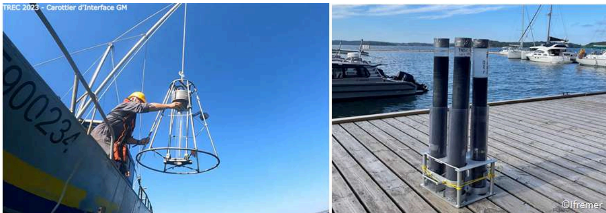
Deployment of the Interface corer for sampling sediment cores to study variations in biodiversity since the beginning of the Industrial Revolution. Raffaele Siano et al, IFREMER.
