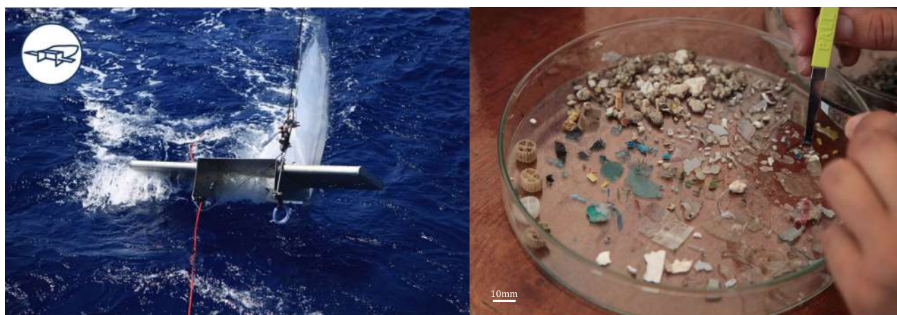
Fig. 2 Photographs of the 330-µm mesh size manta trawl (left) and the following microplastic sorting with sterilized forceps (right) (credit to Noémie Pansiot, Tara Ocean Foundation)
